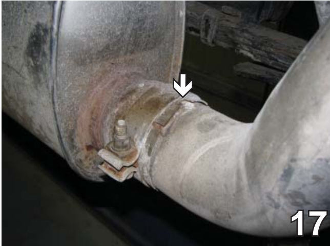
17. Underneath the vehicle on the back side of the muffler, using a 16MM wrench loosen, remove the alignment pin and turn the back tailpipe a little bit.
