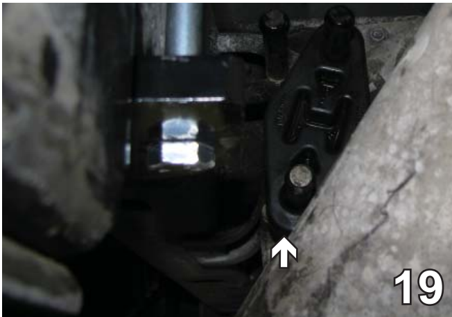
19. Install the new extended rubber on the back. Reinstall the alignment pin and tighten the muffler back up.
