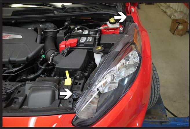
5. Using a T30 Torx, remove the two (2) screws from the headlight. Disconnect the electrical line and set the head light aside. Do this on both sides of the vehicle.
