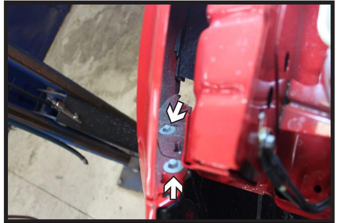
6. Using a 8MM socket, remove the two (2) screws from the edge of the fascia underneath the headlight. Do this on both sides vehicle.
