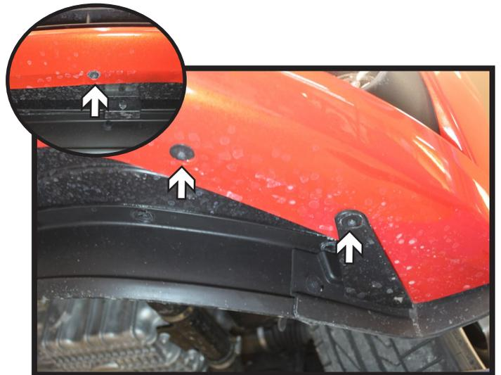
4. Using a 7MM socket, remove the five (5) screws from the underside of the fascia. There are two (2) in each corner and one (1) in the middle.
