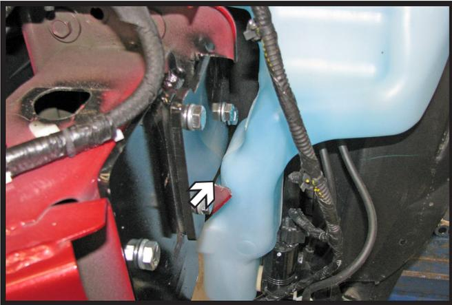
20. Reinstall the washer reservoir. Checking the clearance on the lower part of the reservoir making sure it is not rubbing on the baseplate. It should have minimum 1/16" clearance. If necessary pull the reservoir back and re-tighten the bolts. Reinstall the latch support brace.
