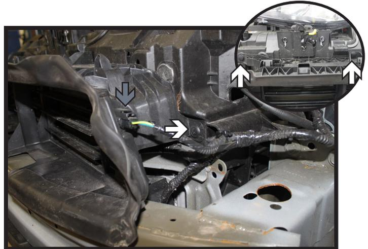
10. **SFE Models:** Remove the four (4) push pins from the shutter shrouding. There is one (1) on each side (white) and two (2) in the middle (inset).
