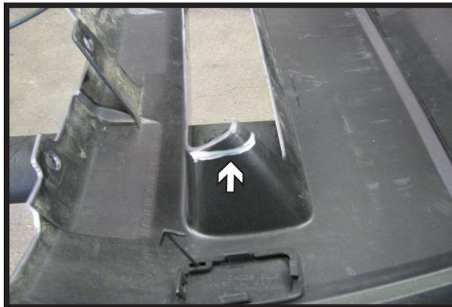
19. Hold the fascia as close to its original position and mark the backside of the fascia, trim as needed. Reinstall the fascia.
