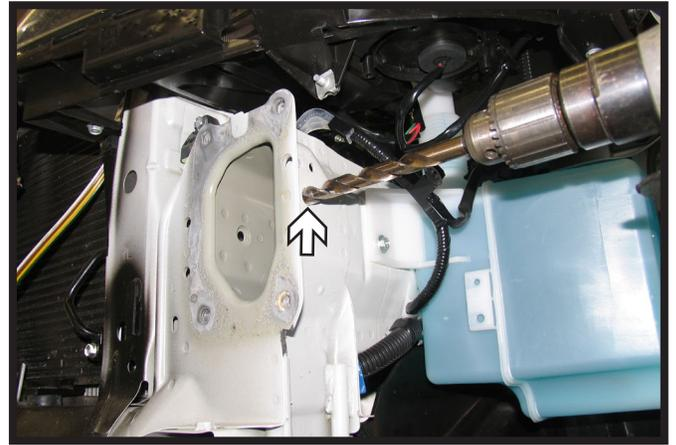
10. Using a 17/32" drill bit, ream out the existing hole in the frame as shown. Do this on both sides of the vehicle.
