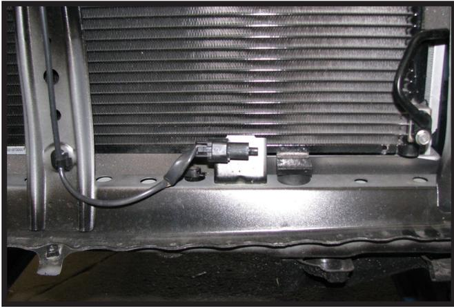
9. Bend the temperature sensor backwards at an angle towards the radiator.
