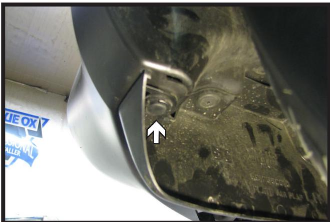
3. Underneath in front of the tire, use a flat screwdriver to remove the push pin in the corner. Do this to both sides of the vehicle.
