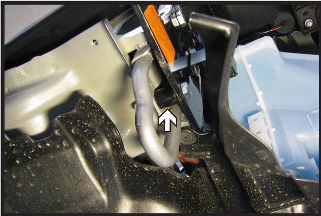
15. On the bottom baseplate hole, insert the spacer tube between the frame and the baseplate. Insert a 3/8"-16 x 2" bolt, 3/8" flat & lock washer and 3/8" lock nut. Do this on both sides of the vehicle.
