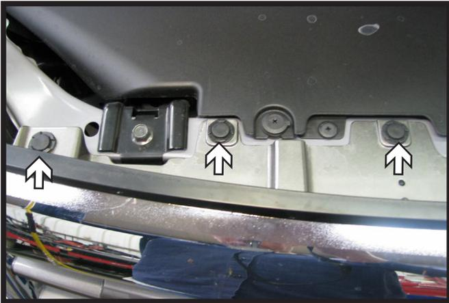
1. Using a flat screwdriver remove the six (6) push pins from the top edge of fascia. There are three (3) on each side.
