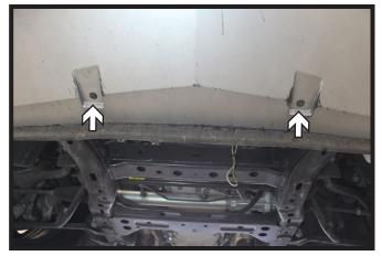
5. Using a 10MM socket, remove the two (2) screws from the underside of the fascia.
