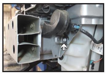
6. Using a 10MM socket, remove the screw from the horn bracket and set the horn aside. Do this on both sides of the vehicle.
