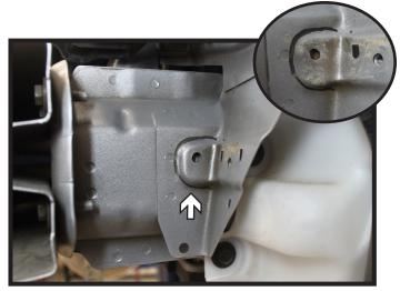
7. Using a hammer, dimple in the front side of the frame protrusion for baseplate installation clearance. Do this on both sides of the vehicle.
