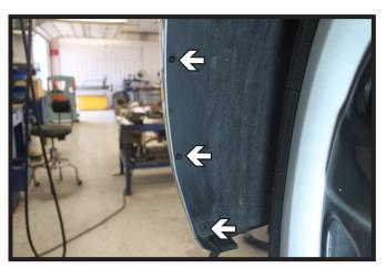
2. In the wheel well, using a T20 Torx, remove the three (3) screws from the outer edge. Do this on both sides of the vehicle.
