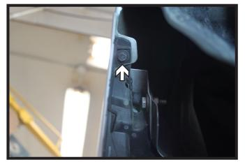
3. Behind the wheel well cover, using a 7MM socket, remove the screw from the fascia joint. Do this on both sides of the vehicle.
