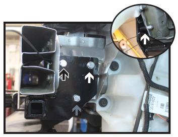
10. Using a 3/8" drill bit, drill the top back hole thru the frame. Install a 3/8"-16 x 1-1/2" bolt with lock washer into the hole and a 3/8" nut plate on the inside of the frame (white). Do this on both sides of the vehicle. Level the baseplate and fully tighten the bolts.
