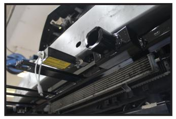
12. **Optional Breakaway**: Using the #10 self drilling screw, attach the bracket to the underside of the bumper in the desired location. Attach the breakaway to the bracket with the supplied 1/4" hardware.
