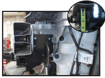
Position the baseplate onto the frame, pulling it tight against the backside of the bumper. Position the bottom of the cross tube approximately 2-3/8" down from the underside of the bumper (inset). Clamp the baseplate to the frame.
