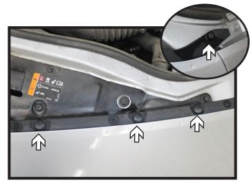
Remove the three (3) push pins just off center of the top of the fascia. Using a 7MM socket, remove the screw from the corner of the top of the fascia (inset). Do this on both sides of the vehicle.
