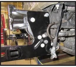
11. Attach the permanent baseplate safety cables to the provided convenience link on the baseplate. The photo above shows the recommended installation of the cables to frame of vehicle. Additional options may interfere with suggested mounting; in this case, secure the cables to a solid piece of the frame as described in the General Information sheet. Be sure the safety cables do not rub against any hoses or moving parts. Do this on **BOTH** sides of the vehicle.
