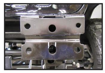
7. Slot the middle bottom hole on the frame as indicated and bend inward to create an access hole. Do this on both sides of the vehicle.
