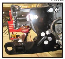
10. **All Models**: Using a 1/2" drill bit, drill the top back hole using the baseplate as a guide. Install the one (1) 1/2" bolt with hardware. Do this on both sides of the vehicle.
