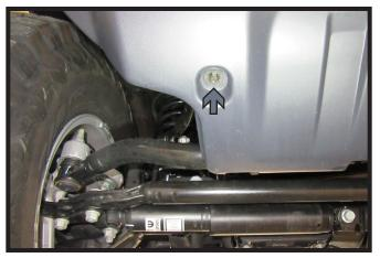
2d. **Overland Models:** Remove the nine (9) push pins from the front edge of the belly pan, there is one (1) in each corner and seven (7) along the center (white). Then using an 8MM socket, remove the two (2) bolts (gray), one (1) on each side, from the belly pan. Remove belly pan and set aside to be reinstalled later.
