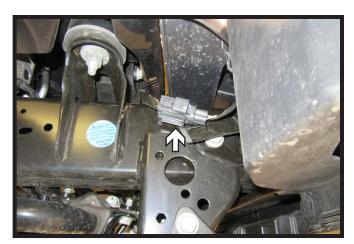
4. Unplug the indicated electrical from the passenger side of the vehicle.
