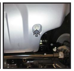
2c. **Sport & Sport S Models:** Remove the eight (8) push pins from the front edge of the belly pan, there are four (4) on each side (white). Then using an 8MM socket, remove the two (2) bolts (gray), one (1) on each side, from the belly pan. Remove belly pan and set aside to be reinstalled later.
