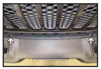
Remove the two (2) push pins, one (1) on each side, from the plastic piece behind the bumper.
