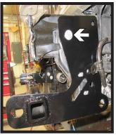
8. Hold frame bracket in place with vice grip (Left). Slide baseplate into position and start the top front 10MM existing bolt with hardware (Right). Ensure that all holes line up and the baseplate is level, then snug down bolt. Do this on both sides of the vehicle.
