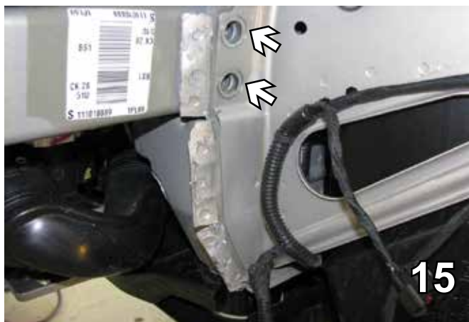
15. Using an 18MM socket and a wrench on the other side, remove the two metric bolts next to the flattened area. Do this on both sides. Set bolts aside to be reinstalled later.
