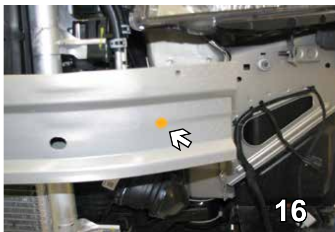
16. Using the 1 1/2" hole saw, drill a hole in the bumper centered with the frame, just in front of the frame end. Do this on both sides.
