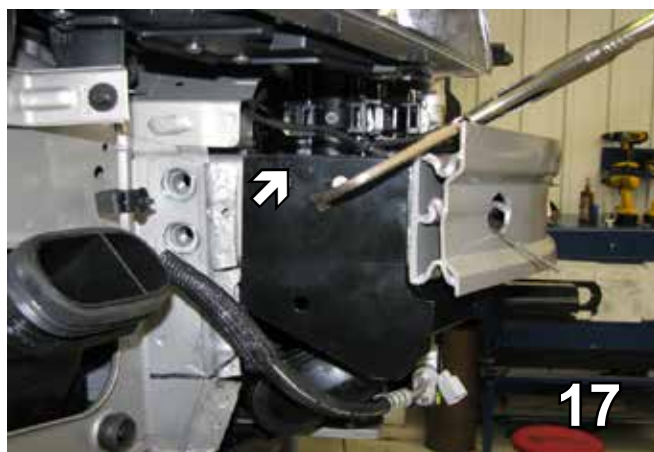
16. Using the 1 1/2" hole saw, drill a hole in the bumper centered with the frame, just in front of the frame end. Do this on both sides.
