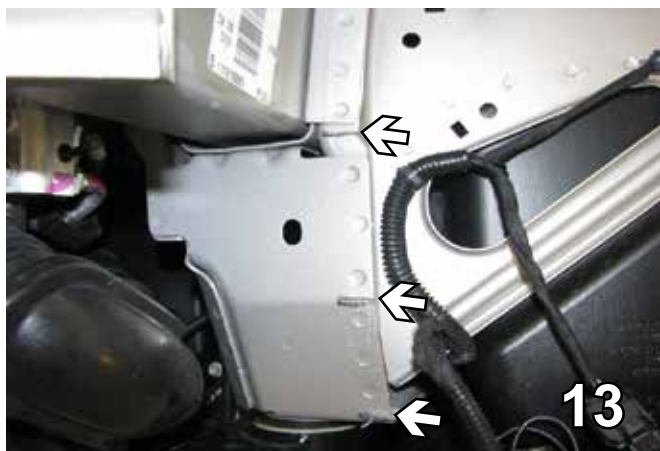
13. Cut frame webbing in these three locations with a reciprocating saw. Do this on both sides.
