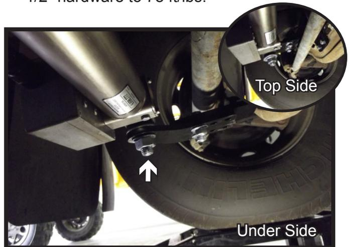
4. Attach the tie rod bracket to the tie rod with the u-bolts and nuts from the appropriate u-bolt kit. DO NOT tighten. Measure the distance from the tie rod to the installation hole. (not shown)
