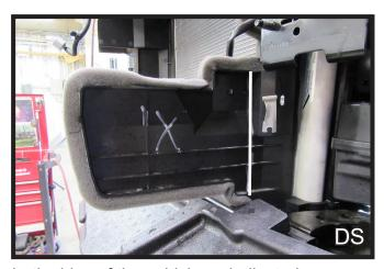
8. Using a utility knife, trim the plastic shielding on both sides of the vehicle as indicated.
