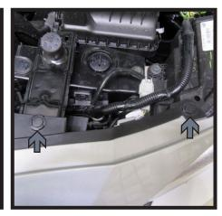
1. Using a 10MM socket, remove the two (2) bolts from the top of the fascia (white). Then remove the four (4) push pins, two (2) on each side (gray)
