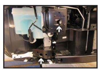
9. Using a 1-1/4" hole saw, drill two (2) access holes. Do this on both sides of the vehicle.
