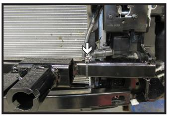
18. Attach the temperature sensor to the baseplate on the driver side of the vehicle using the supplied zip tie.
