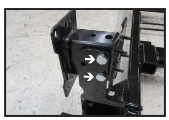
11. Using two (2) 1/2" bolts with hardware, loosely attach the horn extension to the passenger side of the baseplate.
