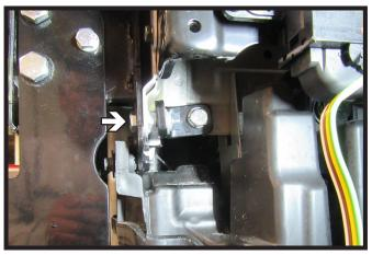
16. Insert the supplied 8MM bolt into the bottom outer hole of the frame extension. Attach hardware and angle bracket. Do this on both sides of the vehicle.
