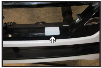
21. **2023-2024 Models**: The bottom black piece on fascia may need to be notched for baseplate clearance. Hold the fascia as close to its original position, mark and trim the fascia around the attachment tabs.
