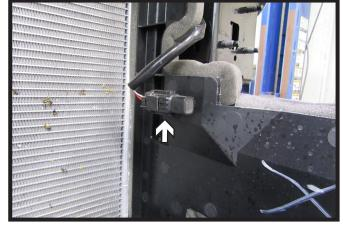
Remove the temperature sensor from the plastic shielding on the driver side of the vehicle. It will be repositioned later.
