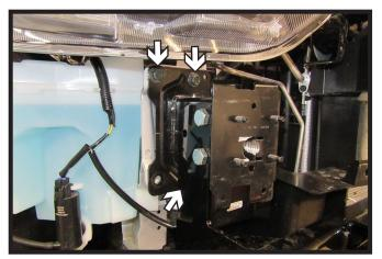
13. Reinstall the horn extension on the passenger side of the vehicle using only three (3) of the existing bolts. The bottom outer bolt on both sides of the vehicle will be installed later using supplied hardware.
