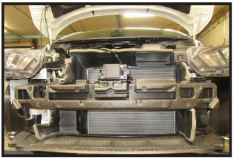
5. Remove the Styrofoam piece from the bumper. It will not be reinstalled.
