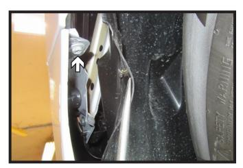
2. Using a flat head screw driver, pull back the wheel well liner. Then using a 10MM socket, remove the one (1) bolt. Do this on both sides of the vehicle.
