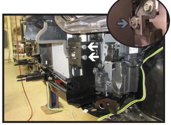
12. Slide the baseplate into place and start the front two (2) 1/2" bolts with hardware on the drive side of the vehicle. Then reinstall the 6MM bolt into the bottom outer hole on the frame extension (inset).
