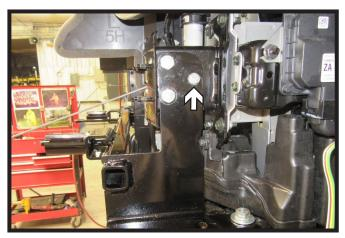
15. Using a 3/8" drill bit, drill the back hole of the baseplate. Install one (1) 3/8" bolt with hardware. Do this on both sides of the vehicle.
