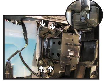
Using a 13MM socket, remove the four (4) bolts (white) from the horn extension on the passenger side of the vehicle.
