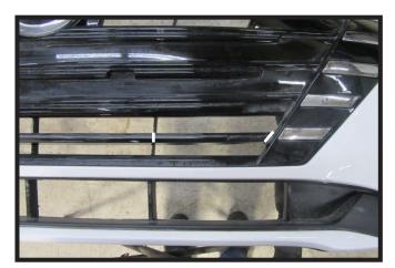
20b. **2023-2024 Models**: Using a reciprocating saw, remove the indicated piece of the fascia to allow room for the baseplate. Do this on both sides of the fascia.
