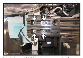
6. Using a 13MM socket, remove the four (4) nuts from the bumper. Do this on both sides of the vehicle. Disconnect push pin on the back side of the bumper on the passenger side of the vehicle. Remove bumper and set aside to be reinstalled later.
