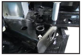
14. Place 1/2" spacer between baseplate and frame. Insert 1/2" bolt with hardware. Do this on both sides of the vehicle. Tighten all hardware at this time
