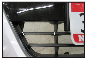
20a. **2020-2022 Models**: Using a reciprocating saw, remove the indicated piece of the fascia to allow room for the baseplate. Do this on both sides of the fascia.
