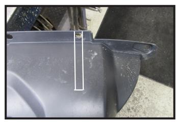
9. Hold the belly pan in place, mark and trim to allow room for the baseplate.
