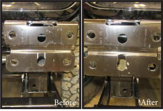
1. Slot the middle bottom hole on the frame as indicated and bend back to create access hole.
