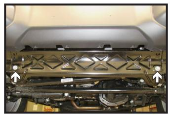
3. Using a 16MM socket, remove the two (2) bolts from the metal guard. Remove and set aside to be reinstalled later.
