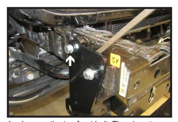
4. Loosen the top front bolt. Then insert spacer plate between the frame and the baseplate. Insert 1/2" bolt into back hole with lock washer and whiz nut. Turn the spacer plate so that it is flush with the baseplate and tighten bolt. Do this on both sides of the vehicle.
