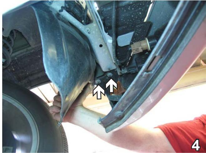
4. Push wheel well cover aside to remove two metric bolts and nuts from the upper corner of fascia using the 10MM socket. Do this to both sides of the vehicle. Set bolts aside to be reinstalled later.
