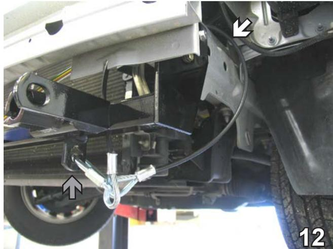
12. Attach the permanent baseplate safety cables to the provided convenience link on the baseplate (see grey arrow). The photo above shows the recommended installation of the cables to frame of vehicle (see white arrow). Additional options may interfere with suggested mounting; in this case secure the cables to a solid piece of the frame as described in the instructions included with the permanent baseplate safety cables. Be sure the safety cables do not rub against any hoses or moving parts.
