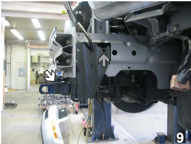
9. Slide baseplate onto the outside of frame rails. Align with upper, existing bolt hole (see grey arrow). The top of the cross tube should be 2 1/4" from the bottom of metal bumper (see white arrow) and the front of baseplate endplate should be resting against the back of the metal bumper bracket. Clamp into place using the vise grips. Do this to both sides of the vehicle.
