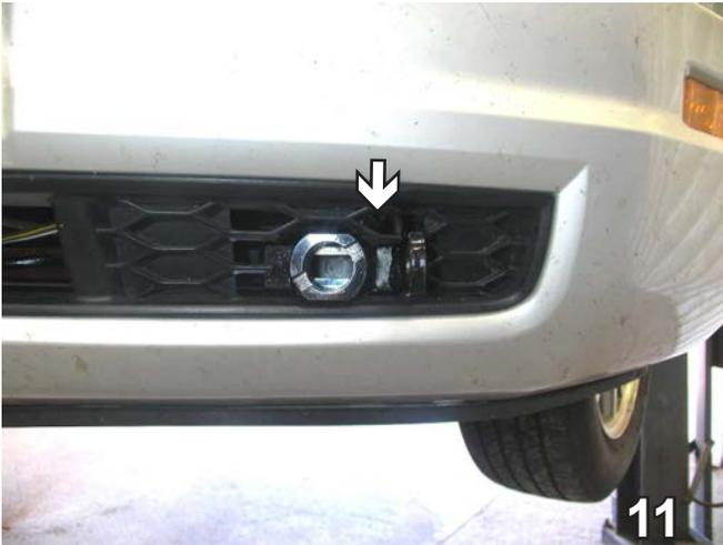
11. Hold fascia up to its original position and, using the side cutters, trim grille style to allow convenience link and attachment tab receiver to come through. Do this to both sides of the vehicle.
