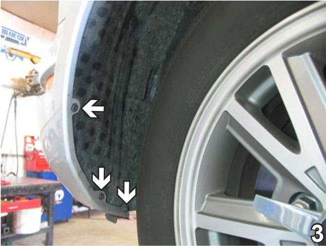
3. Just forward of the front tire, on edge of fascia, remove three Phillips screws. Do this to both sides of the vehicle. Set screws aside to be reinstalled later.
