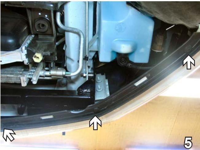
5. Remove seven Phillips pushpins along the bottom of fascia, three each side and one in the center. Pull fascia forward to remove. Set pushpins and fascia aside to be reinstalled later. Passenger's side is shown.
