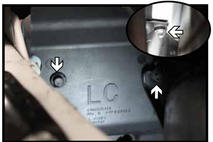
8. On the driver side, remove the two (2) push pins from the plastic shrouding. Then using a 7MM socket, remove the screw from behind the air baffle. Set the air baffle aside.
