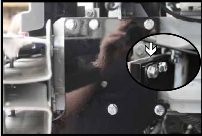
16. Using a 13/32" drill bit, drill the top three (3) holes and bottom two (2) holes into the frame. Install a 3/8"-16 x 1-3/4" bolt, 3/8" lock washer and 3/8"-16 nut into the each of the holes. On the top holes use the spacer plate between the frame and baseplate. Tighten down all fasteners. Do this on both sides of the vehicle.
