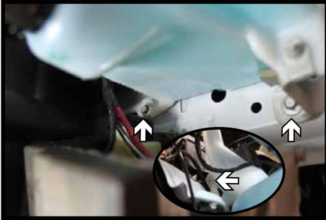
12. Using a 10MM socket, remove the two (2) screws from the bottom side of the washer reservoir. Then remove the upper screw, disconnect lines and set the reservoir aside.
