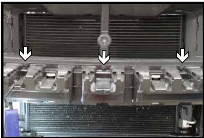
7. Remove the three (3) push pins from the plastic fascia support and unsnap from the metal bumper.
