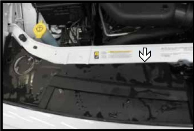
1. Lift up and remove the plastic radiator covers from both the passenger and driver side of the vehicle.
