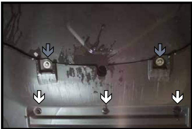
10. On the underside of the vehicle remove the plastic sheilding. Remove the three (3) push pins (white). Then using a 10MM socket, remove the two (2) bolts (gray).
