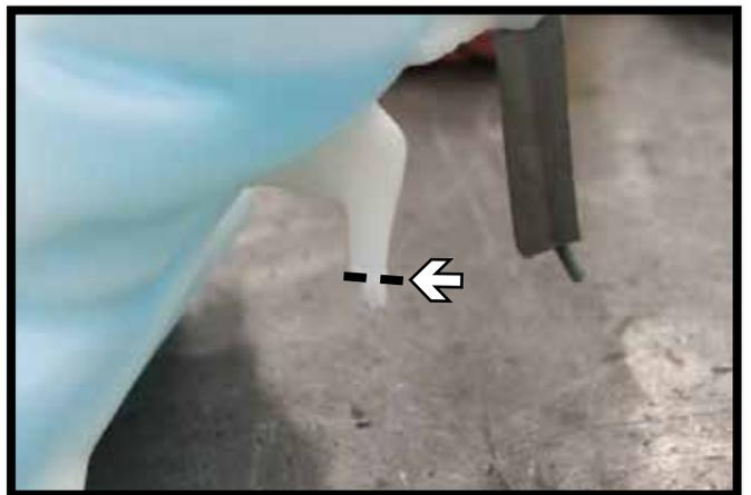
19. Trim the plastic peg off the washer reservoir. Reinstall the reservoir with the supplied 6MM bolts and spacers. Reattach the power steering pump.
