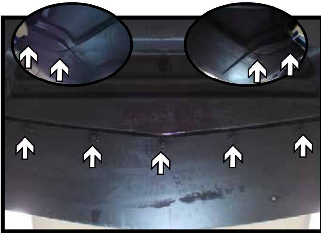
5. Using a 7MM socket, remove the nine (9) screws from the bottom edge of the fascia. There are two (2) on each side and five (5) in the center.
