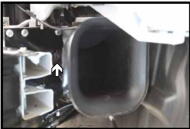
18. Reinstall the air baffle, using the existing hole thru the baseplate.
