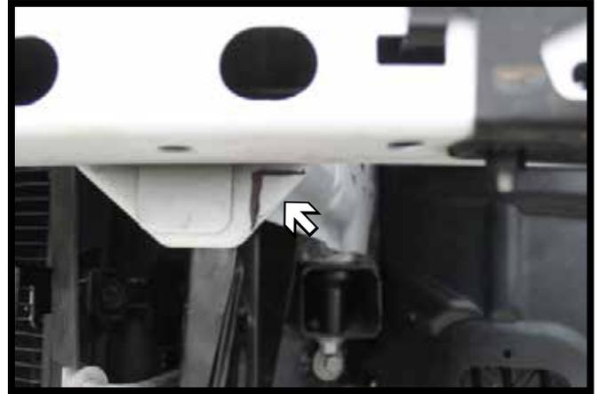
13. Using a reciprocating saw, notch the frame end flush with the bottom of the bumper and flush with the outside of the frame. Do this on both sides of the vehicle.
