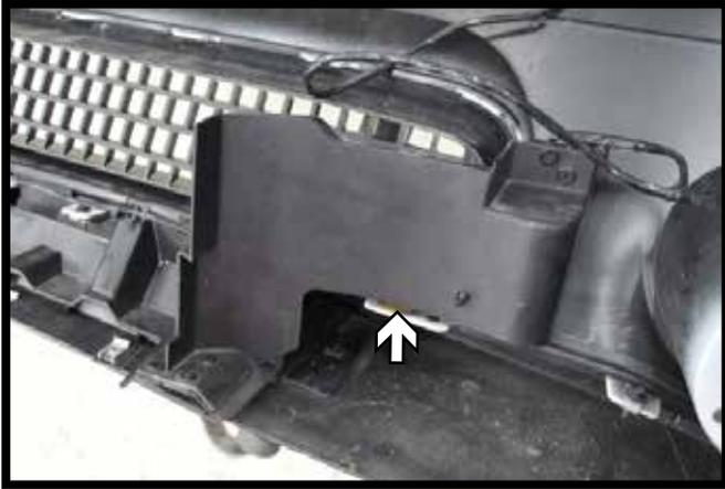
20. Before reinstalling the fascia, remove the plastic sheilding from both sides by removing the plastic rivets.
