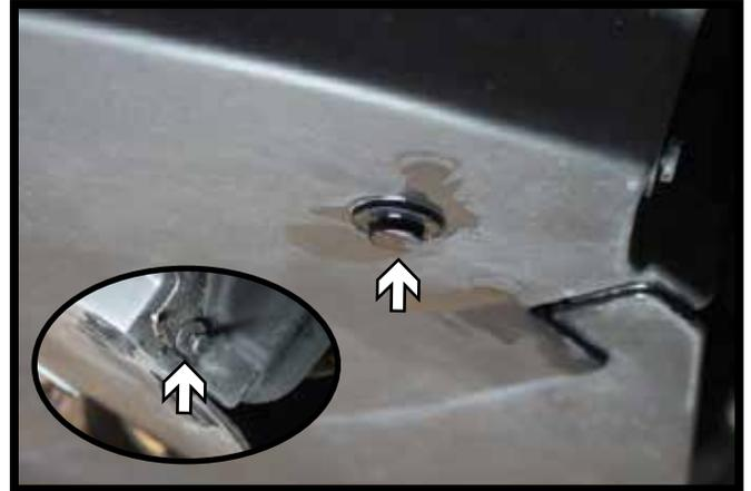
9. Remove the plastic shrouding on the driver side. On the top side, remove the rear push pin and the upper push pin (left). On the underside of the shrouding, remove the bottom push pin and the push pin located just inside the wheel well (right)
