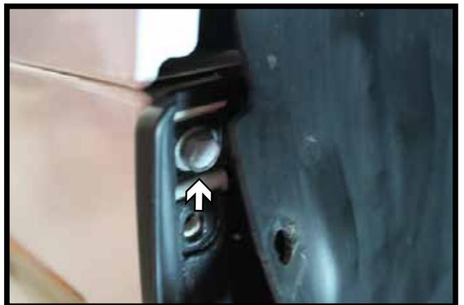
4. Using a 10MM socket, remove the screw from behind the wheel well cover at the top edge of the fascia. Do this on both sides of the vehicle.
