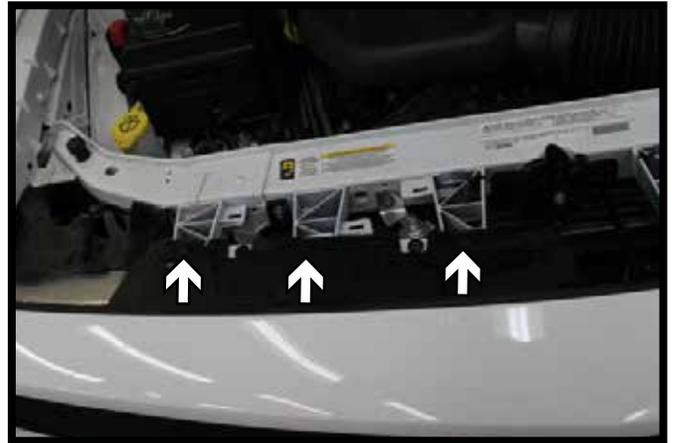
2. Remove the six (6) push pins from the top side of the fascia. Three (3) push pins from both sides of the vehicle.
