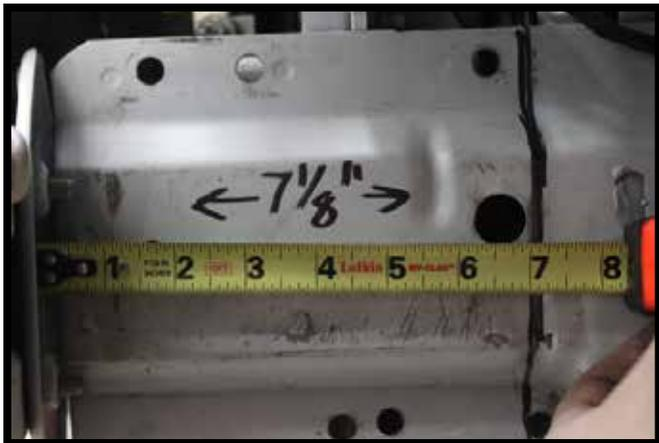
14. Measure back from the backside of the frame end plate 7-1/8" and make a mark. Do this on both sides of the vehicle.
