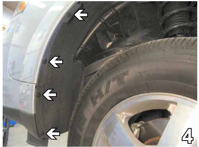
4. All Models: Remove four pushpins inside the wheel well, just forward of the front tires. Do this to both sides of the vehicle. Set the pushpins aside to be reinstalled later.
