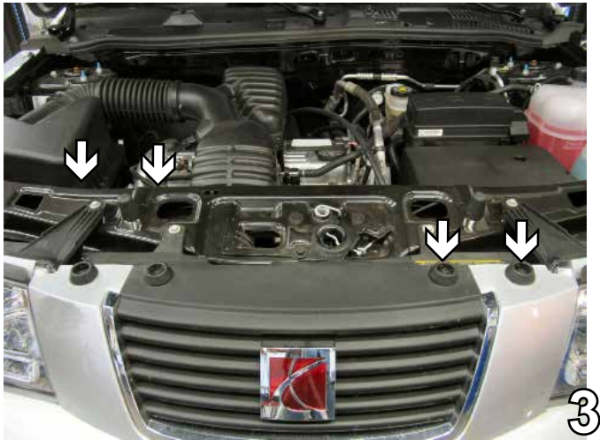
3. 2006 Models ONLY: Remove four metric bolts from the top edge of the fascia with the 10MM socket. Set the metric bolts aside to be reinstalled later.
