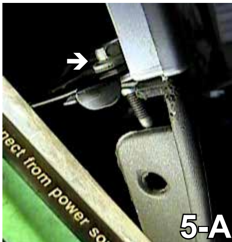
5. All Models: Using the 10MM socket, remove the metric bolt on the fascia corner. Do this to both sides of the vehicle. (5-A is the 2002-05 models and 5-B is the 2006 model). Set the bolts aside to be reinstalled later.
