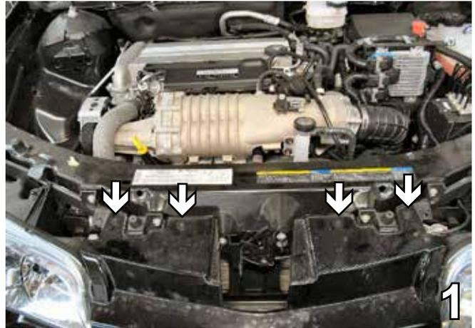
1. Using a 7MM socket, remove four metric bolts from the top side of the fascia. Set bolts aside to be reinstalled later.
