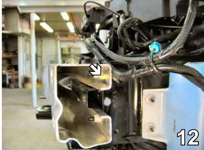
12. Release Christmas tree clip to move electrical cable out of the way for drilling.
