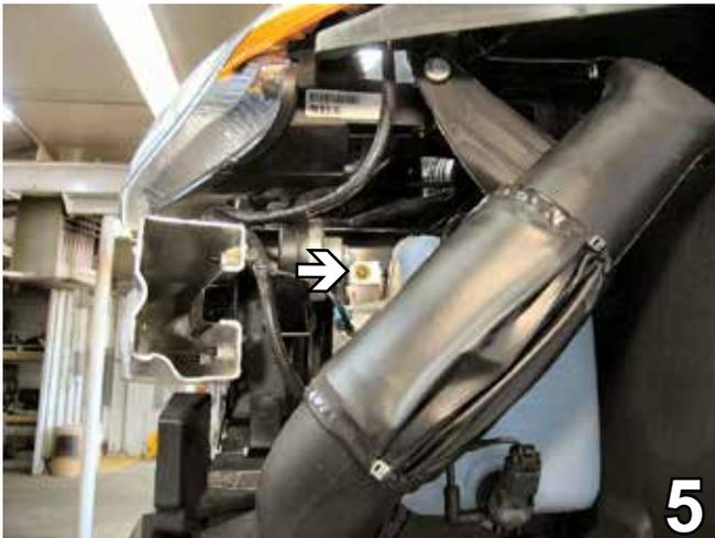
5. Using a 10MM socket, remove one metric bolt from the horn bracket. Disconnect the horn and bracket. Set all aside to be reinstalled later. Do this to both sides of the vehicle.
