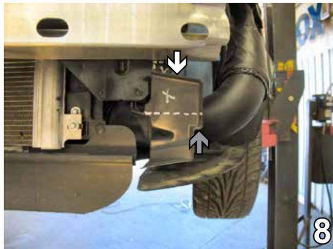
8. Mark and trim away air dam 1" up from the bottom corner, see the grey arrow in the photo above. Do this to both sides of the vehicle.
