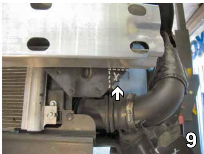
9. Using the reciprocating saw, cut the webbing under the metal bumper. Cut flush with the bottom of the bumper and the frame rail edge. Do this to both sides of the vehicle.
