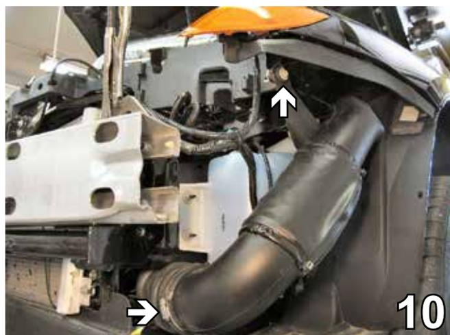
10. Using a 1/4" socket, loosen up the clamp on the air intake tube. Using a 10MM socket, remove the metric bolt securing the tube. Remove the air intake tube and set aside with bolt and clamp to be reinstalled later.
