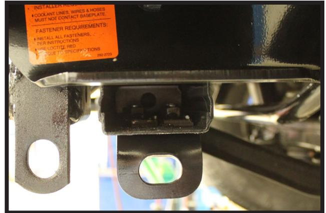
11. Attach the appropriate convenience link to the bottom of each side of the frame as indicated using two (2) 12MM bolts with 12MM lock washers and 1/2" nut plates.
