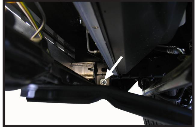
6. Tilt the back of the baseplate down, slide cross tube between the tie down loops and the tab. Align the forward hole of the baseplate with the existing hole of the lower extension that has the 7/8" O.D. spacer tube inserted. Place the 1/2" x 4" hex bolts through the outside of the baseplate and hand tighten.
