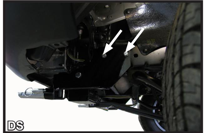
8. Insert 3/8"-16 x 2" bolts with 3/8" lock washers into the holes from the outside of the frame.
