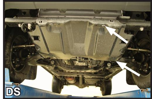
1. Using a 12MM socket remove the four (4) bolts, two (2) per side, from the belly pan and set aside for reinstalling after baseplate installation.
