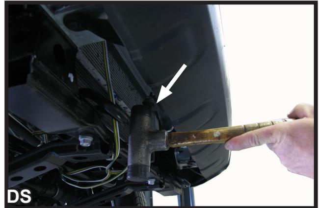
4. Remove the two (2) push pins from the bottom edge of the front fascia. After removing the push pins, use a rubber mallet to bend the tabs upward where the push pins were located. This will prepare the opening for the baseplate installation.
