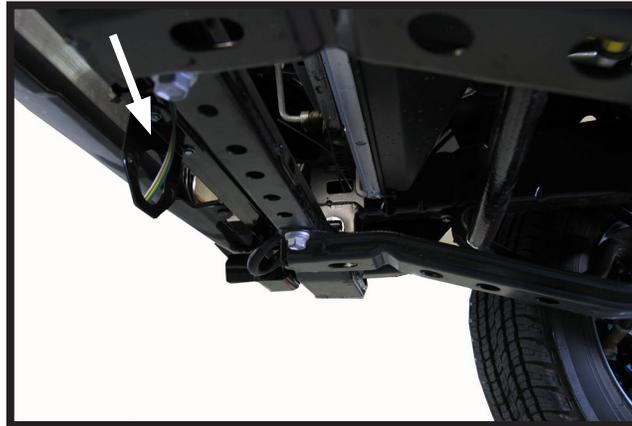
10. Align the electrical bracket with the center of baseplate cross tube, install the self tapping screws into the bottom of cross tube with the 5/16" nut driver and drill. Reposition tabs to their original placement and reinstall push pins.
