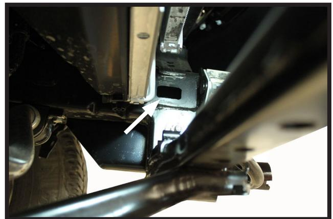
9. On the inside of the frame, remove the cap on BOTH sides of the vehicle. Install 3/8-16 nut plates onto the 3/8" x 2" bolts from step #8. Fully tighten all bolts and reinstall the caps.
