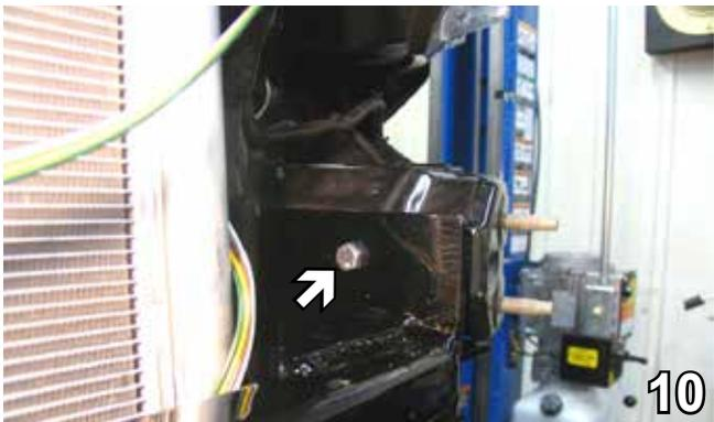
10. Insert 3/8-16 x 1 1/4" hex bolts with 3/8" lock washers attached to 3/8-16 nut plates with 14" wire inserted into the frame rail on both sides to hold the baseplate in place.
