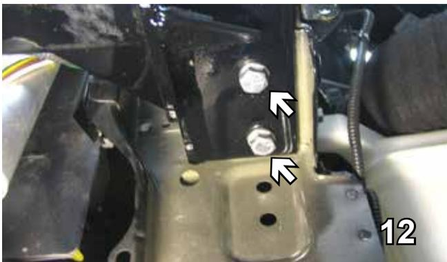
12. Insert 3/8-16 x 1 1/4" hex bolts and 3/8" lock washers with 3/8-16 nut plates with 14" wire inserted into the frame rail. Use loctite on all the bolts and tighten. Do this on both sides and the bolts inserted previously.
