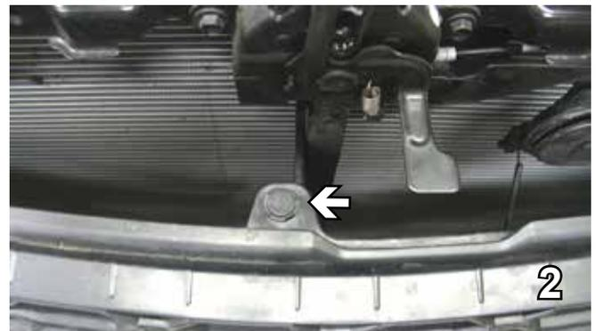
2. Remove push pin from top edge of fascia just below hood latch and set aside for reinstallation later.
