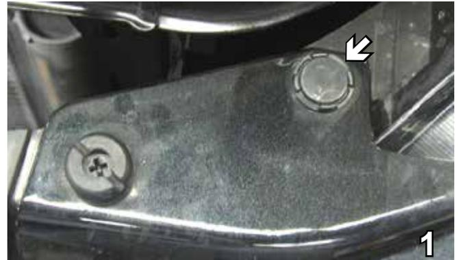
1. Remove push pins (white arrow) from the top corner edge of the fascia. Using the Phillips screw driver, remove the Phillips screw (gray arrow), do this to both sides and set aside for later reinstallation.
