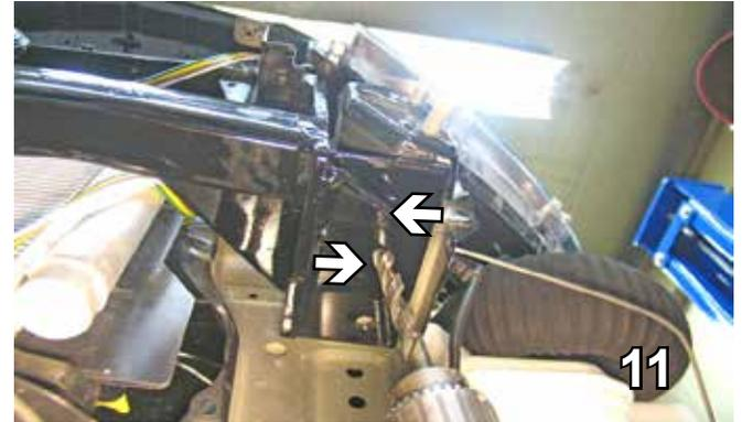
11. Using the baseplate as a template, drill both holes in the under side of the frame rail with a 13/32" drill bit. Do this on both sides.
