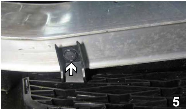
5. Behind the fascia on the bottom of the bumper, are two push pins to remove from the fascia's tabs. Remove with a flat screw driver. Pull the fascia forward on both sides and set aside carefully for later reinstallation.
