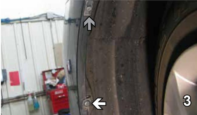
3. Just forward the front tire on the upper corner of the fascia and inside the wheel well, turn the screw 90° to remove it (white arrow). Using a Phillips screw driver, remove the upper screw (gray arrow). Do this on both sides and set aside for reinstallation later reinstallation.
