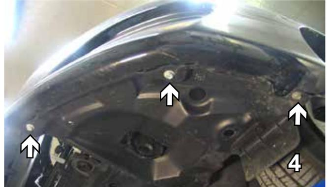
4. Just forward of the front tire underneath the bumper, using a 10MM socket, remove the three metric bolts. Do this on both sides and set aside bolts for later reinstallation.
