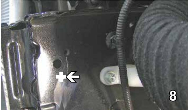
8. Drill a hole in the frame rail under but connected with the existing hole using the 1 1/4" hole saw on both sides. This hole will allow the installer to insert the nut plates inside of the frame rail.
