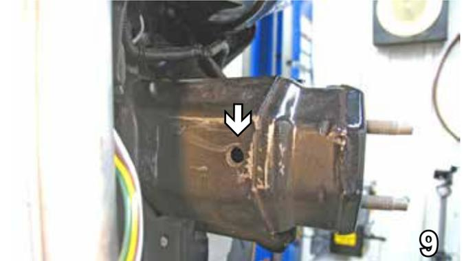
9. Slide the baseplate up between the frame rails and align with the existing hole on each side.
