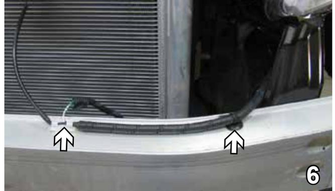
6. On the driver's side only, using a flat screw driver release the tabs from the top of the bumper and tie the wire loom up in the open area during baseplate installation.
