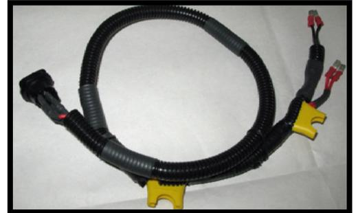
The Fuse ByPass Switch is designed to be mounted in the upper rear of the floor console beside the power outlet. If the vehicle is equipped with the optional audio/video connections, then the switch should be mounted below these connectors on the rear panel of the console. The wiring will flow down behind the console rear panel, then fed under the floor carpet to the under floor battery compartment and make connection with the two fuse holders found in the wiring.
