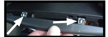
4. Remove the rear panel of the console using your fingers at the bottom and sides where the side panels meet the rear panel and carefully pull out the panel. The rear panel is attached by push pins near the top and bottom on the side panels. The upper corners also have tabs that fit under the top section of the console. Gently pry until the rear panel comes loose and disengage the upper tabs to remove completely remove the panel.
