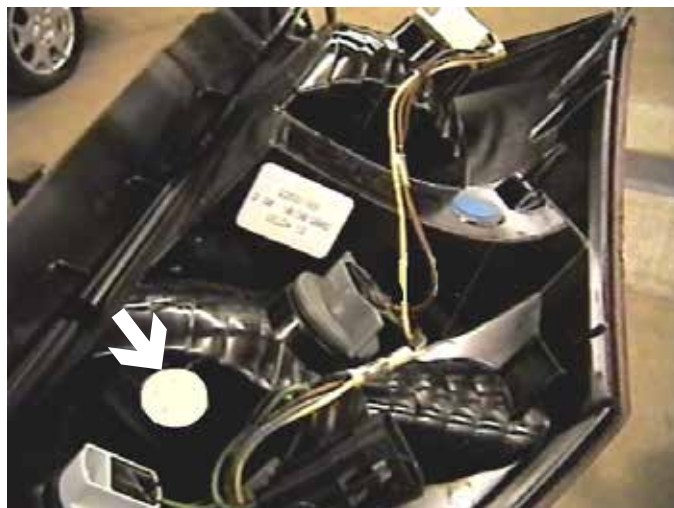
Location of BX8869 bulb and socket installation on driver's side (right photo).
