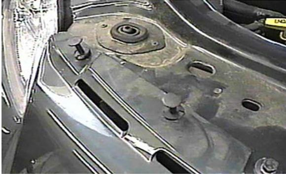
1. Remove the six push pins from the top of grill.
