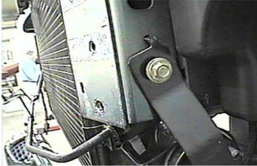
7. Unplug electrical connection from horn and remove horn bracket with a 10MM socket, set aside. Factory horn bracket will not be reused.
