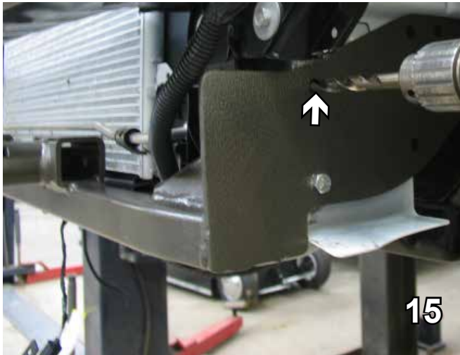
15. Using the baseplate as a template, drill six holes with a 13/32" drill bit.
