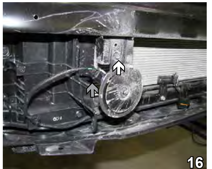
16. Using the 10MM socket, remove the bolt attaching the horn to the bracket (white arrow). Unplug the horn (gray arrow).
