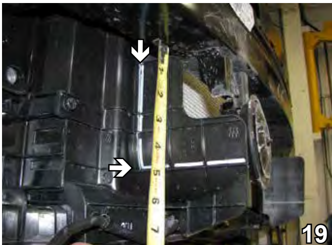
19. On the passenger side, cut the plastic 5" straight down and across along the ridge.
