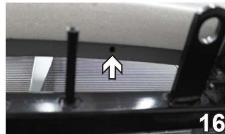
14. On the passenger side, the back bolt (white arrow) is a 3/8-16 x 1" hex bolt and 3/8" lock washer with 3/8-16 hex nut. The front two (grey arrows) are 3/8-16 x 1 1/2" hex bolts with 3/8" lock washers and 1/4" x 1" x 1" nut plates inserted through the opening above the baseplate. Tighten all bolts with Loctite Red.
