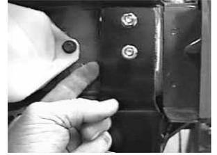
11. Drill the two 3/8" holes for each side plate, use baseplate as a template. Place spacer plates between the sideplates and frame and use hardware as shown in the diagram on last page. NOTE: The fluid reservoir bolts may need to be removed to insert the spacer for the passenger side.
