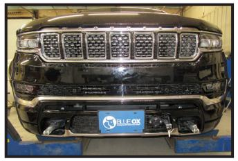
21. Hold the fascia as close to its original position, mark and trim the fascia around electrical rods. Reinstall the fascia and reconnect all electrical connections and hose.
