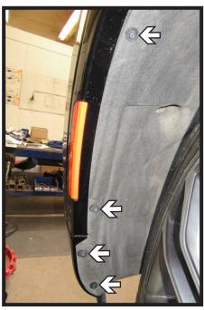
Using an 8MM socket, remove the four (4) bolts from the wheel well edge. Do this on both sides of the vehicle.
