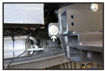
14. Attach support bracket to baseplate using one (1) 1/2" x 1-1/2" bolt with flat washer and nylon lock nut. Do this on both sides of the vehicle.
