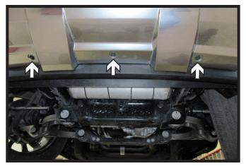
4. Using a 10MM socket, remove the three (3) bolts from the bottom of the fascia.
