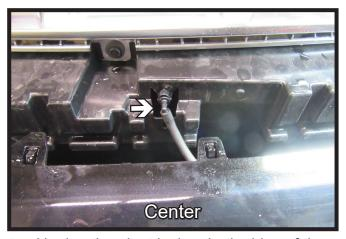
5. Remove fascia and set aside to be reinstalled later. Unplug the electrical on both sides of the vehicle and hose in the center as the fascia is removed.
