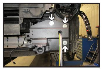
13. Hold baseplate in place and start the three (3) 1/2" x 1-1/2" bolts with flat washers and nylon lock nuts. Snug up the baseplate into place but leave loose. Do this on both sides of the vehicle.
