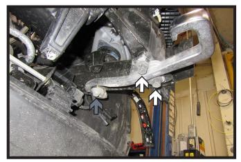
5. Using a 21MM socket, remove the front two (2) bolts (white) on the tow hooks. Then using an 18MM socket, remove the back one (1) bolt (gray). Remove tow hook, it will not be reinstalled. Reinstall back bolt from tow hook (gray). Do this on both sides of the vehicle.
