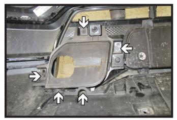
Using a 7MM socket, remove the six
