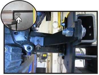
15. Using a 1/2" drill bit, drill the bottom inside hole on the front of the baseplate (inset). Then using the support bracket as a template, drill 1/2" hole in frame (gray). Do this on both sides of the vehicle.
