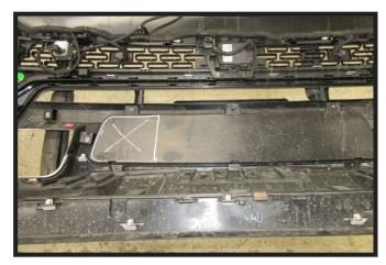
10. Using a reciprocating saw, remove the indicated area from the driver side of the plastic piece on the back of the fascia.
