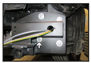
17. Install one (1) 1/2" x 1-1/2" bolt with flat washer and nylon lock nuts into the bottom inside hole on the front of the baseplate. Leave loose at this time. Do this on both sides of the vehicle.
